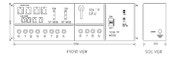
Fig. Tentative layout of the Sub distribution Board
